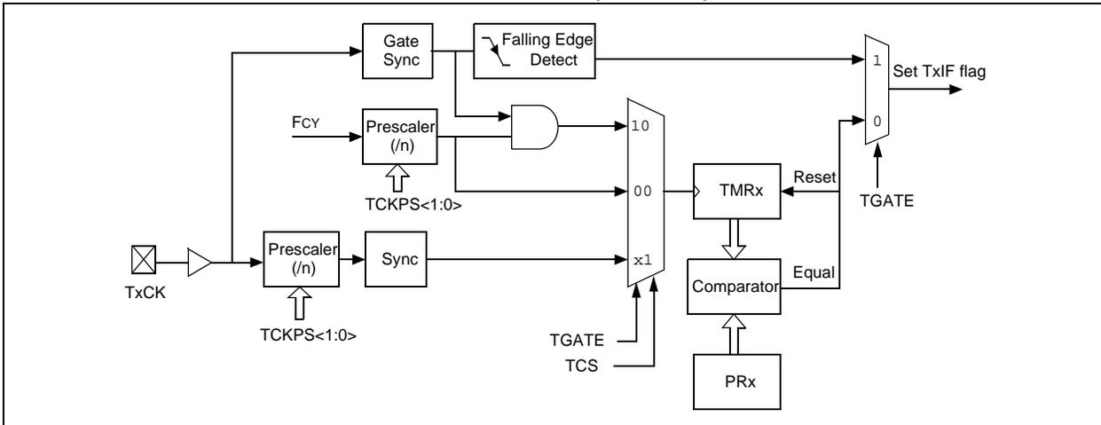
**FIGURE 13-2: TYPE C TIMER BLOCK DIAGRAM (x = 3 or 5)**
