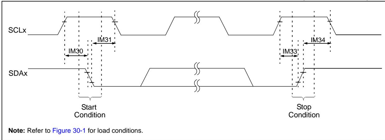
FIGURE 30-18: I2Cx BUS DATA TIMING CHARACTERISTICS (MASTER MODE)
