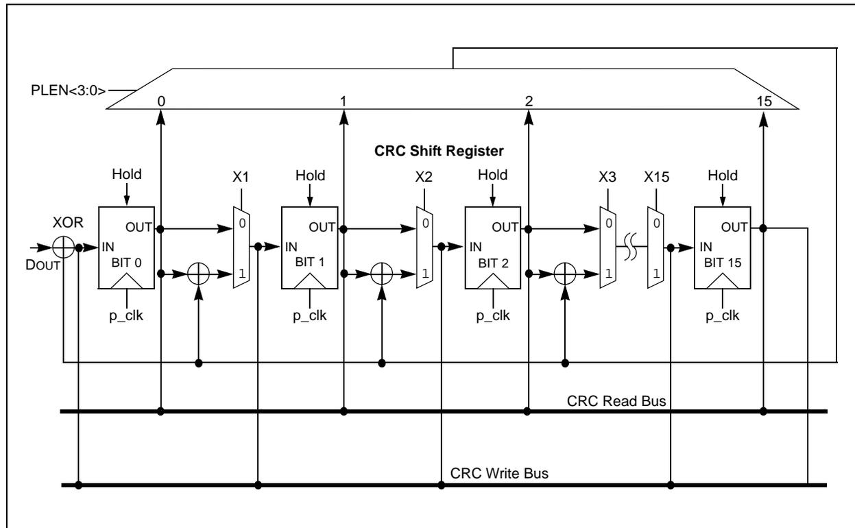
FIGURE 25-2: CRC GENERATOR RECONFIGURED FOR  $x^{16} + x^{12} + x^5 + 1$
