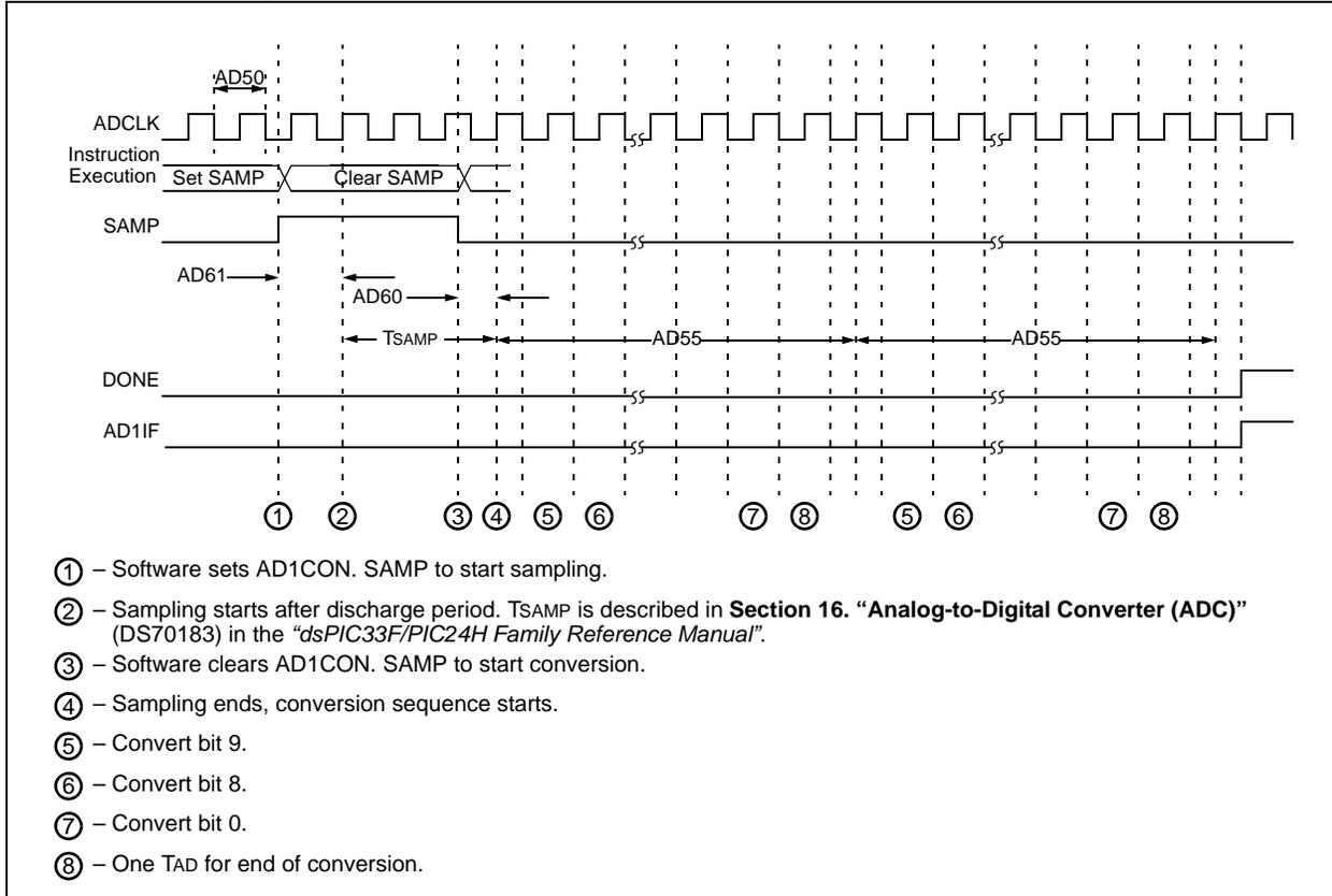
**FIGURE 30-26: ADC CONVERSION (10-BIT MODE) TIMING CHARACTERISTICS (CHPS<1:0> = 01, SIMSAM = 0, ASAM = 1, SSRC<2:0> = 111, SAMC<4:0> = 00001)**
