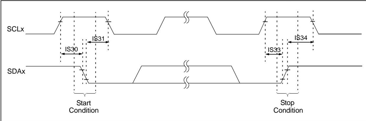
**FIGURE 30-20: I2Cx BUS DATA TIMING CHARACTERISTICS (SLAVE MODE)**
