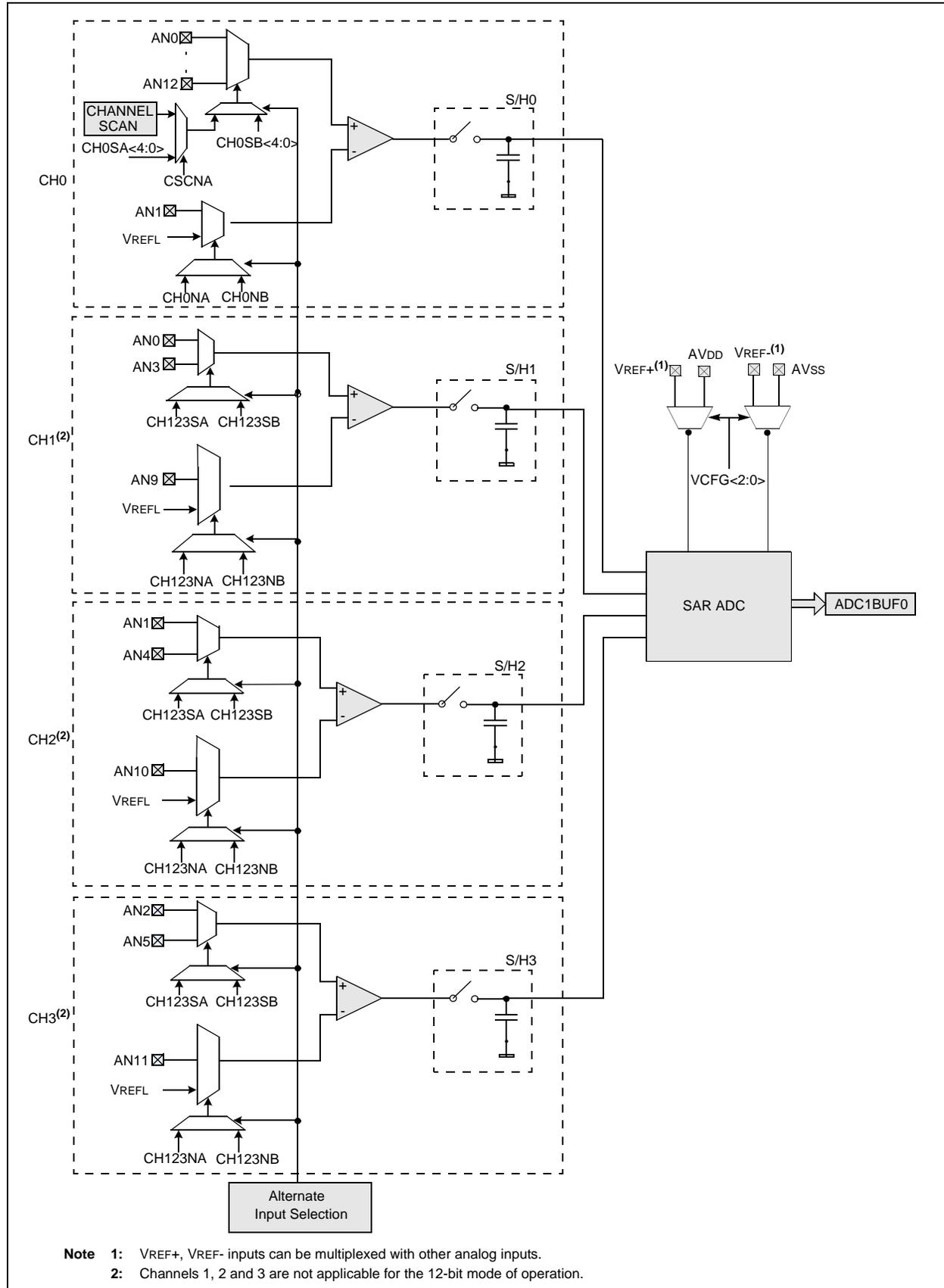
FIGURE 21-3: ADC CONVERSION CLOCK PERIOD BLOCK DIAGRAM
