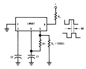
Connect Pin 3 to 2.8V to Invert Output
