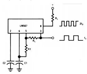
Figure 16. Oscillator with Double Frequency Output
