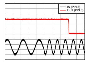
Figure 13. Frequency Detection
