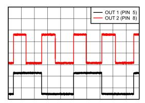
Figure 17. Double Frequency Output
