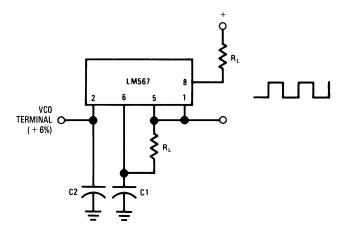
Figure 18. Precision Oscillator Drive 100-mA Loads
