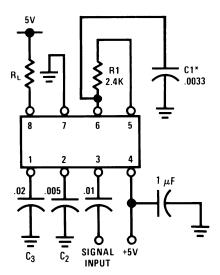
$f_i$  = 100 kHz + 5 V \*Note: Adjust for  $f_o$  = 100 kHz.
