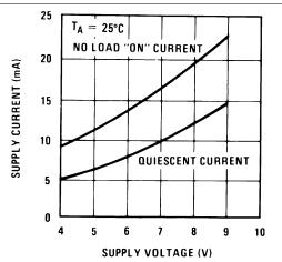
Figure 8. Typical Supply Current vs Supply Voltage
