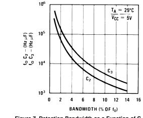
Figure 7. Detection Bandwidth as a Function of C2 and C3
