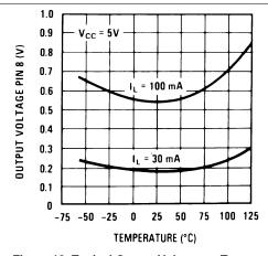
Figure 10. Typical Output Voltage vs Temperature
