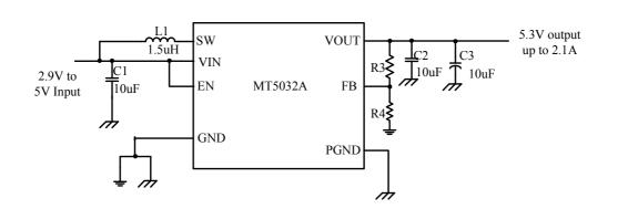
Figure 1. MT5032A Typical Application Circuit
