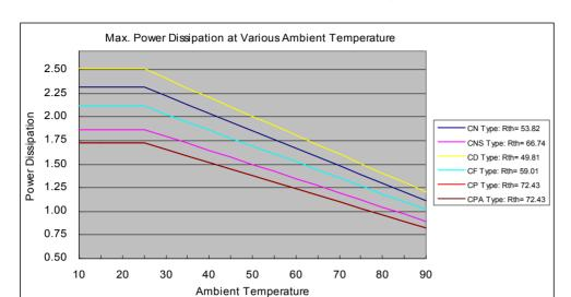
The maximum power dissipation,  $P_D(max) = (Tj - Ta) / R_{th(j-a)}$ , decreases as the ambient temperature increases.
