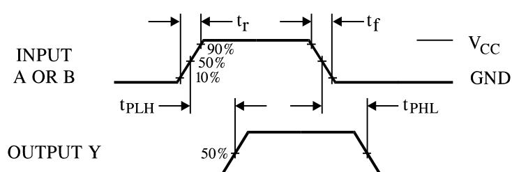
**Figure 1. Switching Waveforms**
