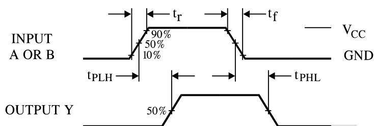
**Figure 1. Switching Waveforms**
