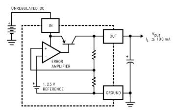
Figure 33. LP2950-N Functional Block Diagram
