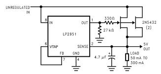
Figure 44. 300-mA Regulator with 0.75-V Dropout
