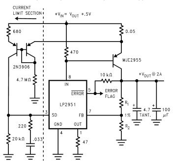
Figure 50. 2-A Low Dropout Regulator
