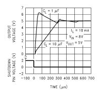
Figure 38. LP2951-N Enable Transient
