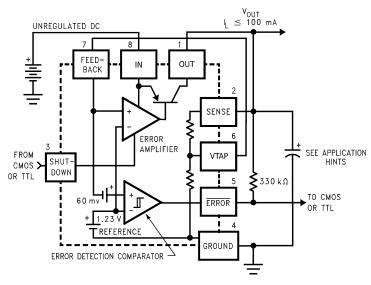
Figure 34. LP2951-N Functional Block Diagram
