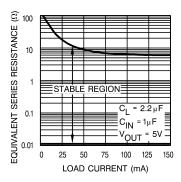
Figure 37. Output Capacitor ESR Range
