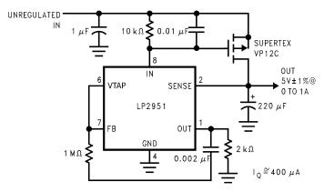
Figure 36. 1-A Regulator with 1.2-V Dropout
