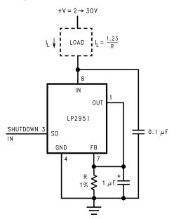
Figure 46. Low Drift Current Source
